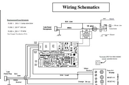
Connect circuit for 120-vac Range outlet @ Posts 1 and 2 where required by application.
